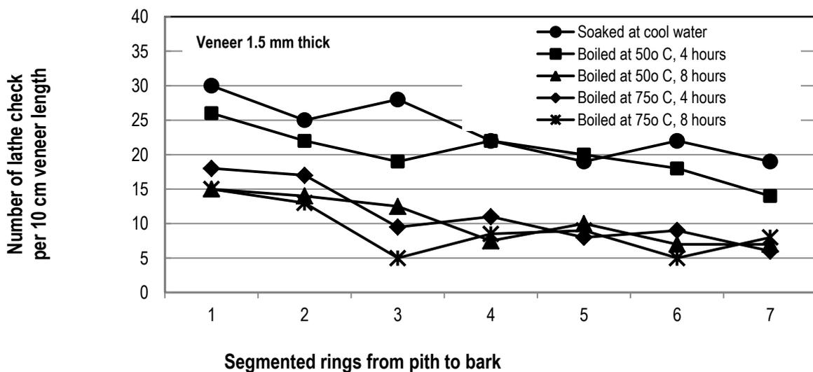
**Fig. 2.2** - Variation of lathe check frequency from pith to bark for the 1.5 mm veneer thickness
