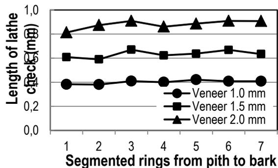
**Fig. 2.5** - The progress of length of lathe check from pith to bark
