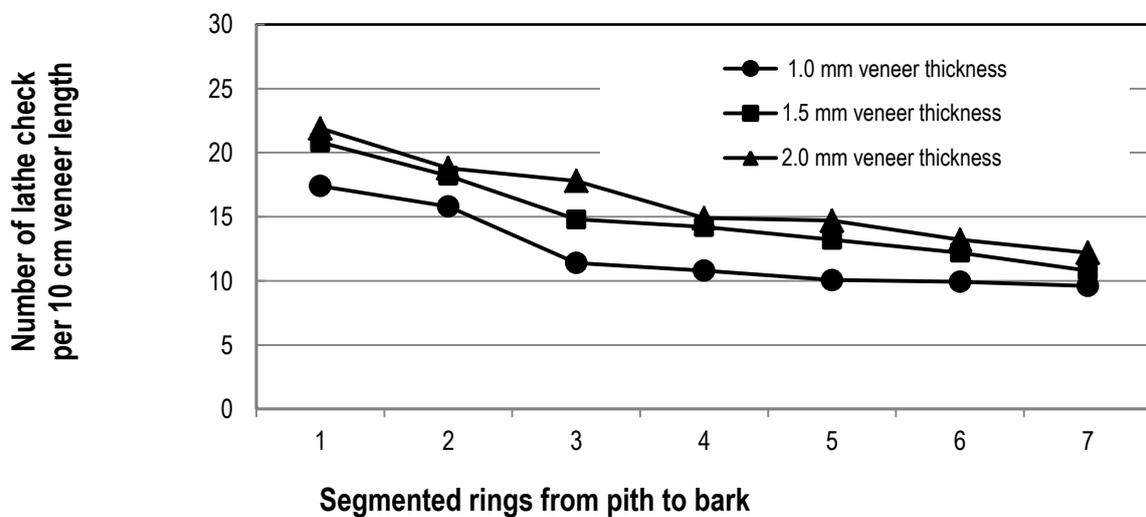
**Fig. 2.3** - The effect of veneer thickness on the frequency of lathe checks
