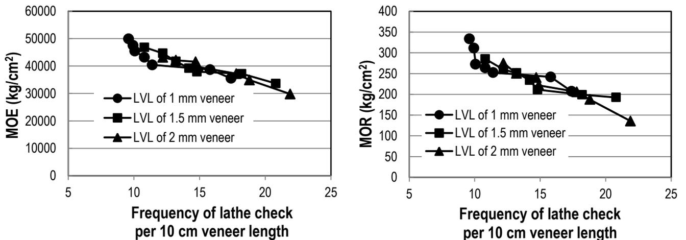
**Fig. 2.7** – The effect of lathe check on the bending strength (MOE and MOR) for different veneer thickness
