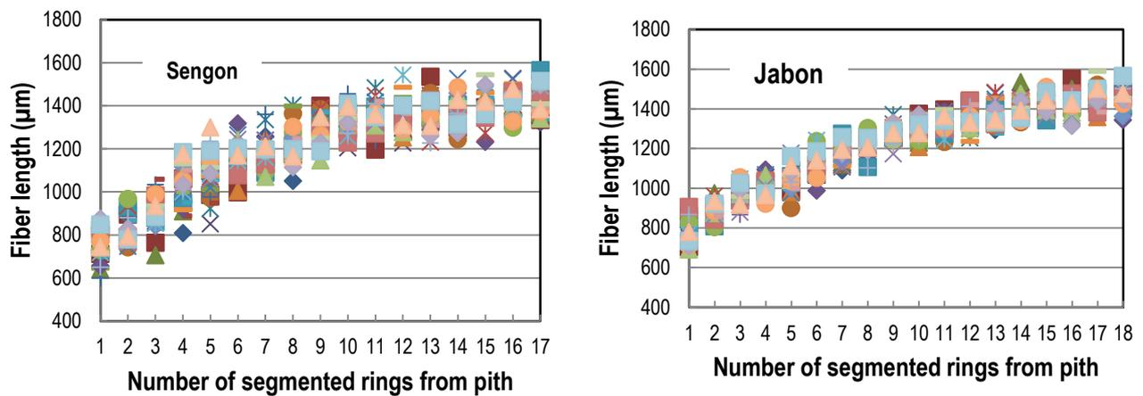
**Fig. 1.3** Profiles of fiber length from pith to bark for sengon and jabon
