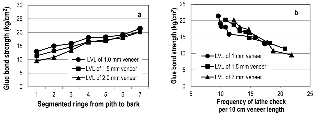
Fig. 2.6 – The effect of juvenility and lathe check on the glue bond strength for different veneer thickness
