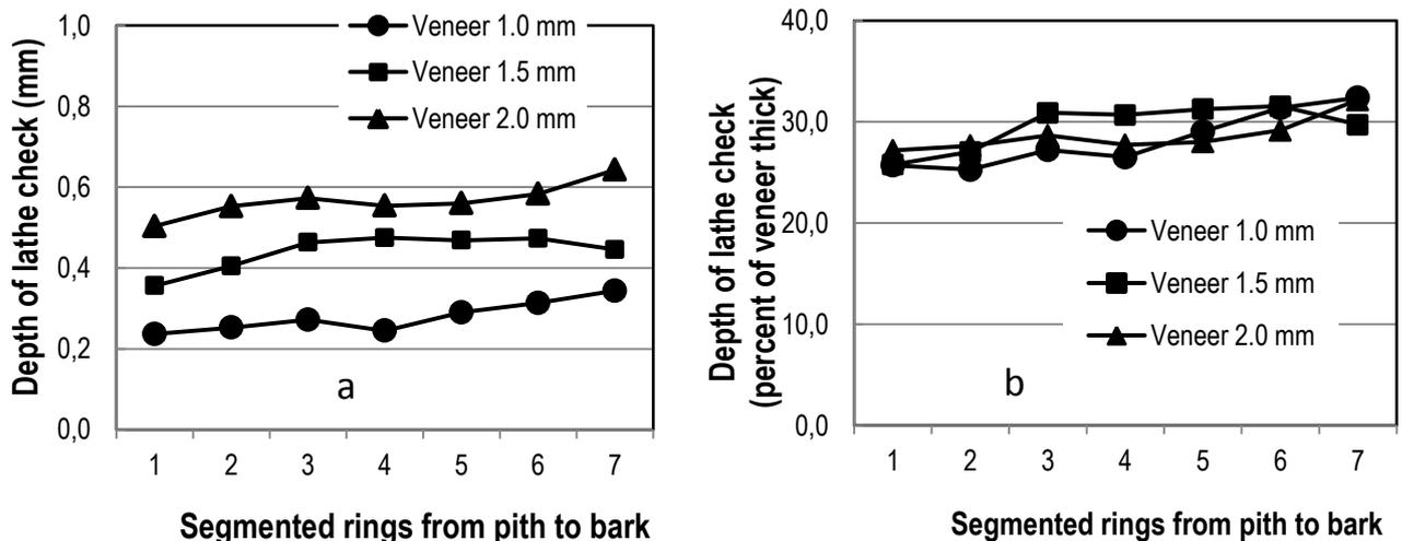
**Fig. 2.4** - The progress of depth of lathe check from pith to bark
